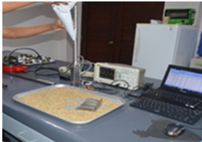
Figure 3. Calibration tests conducted for grain probe moisture meter
